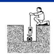
NC2 vertical, direct, unobstructed access with continuous attachment to a man riding hoist or similar mechanical rescue device.
