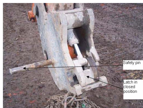
Semi automatic quick hitch (safety pin about to be inserted)
